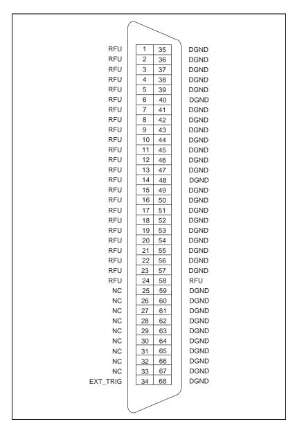
Figure 1-5. SHC50-68 68-Pin Connector Pin Assignments
